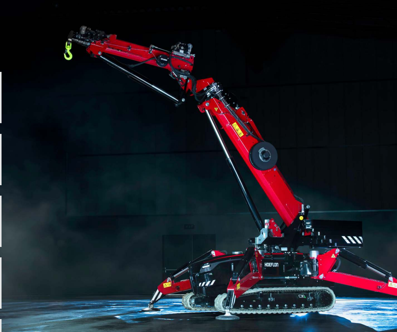
Adjustable section with manual jib extension
