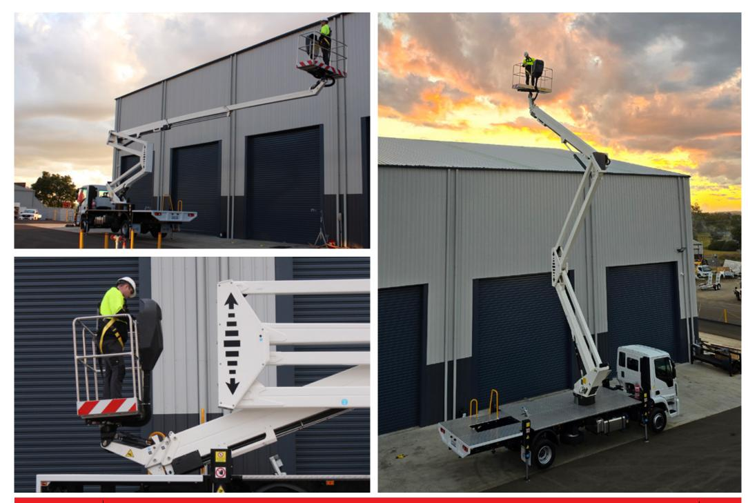
"Plumb line" vertical plane movement with the double articulating pantograph boom ideal for cleaning facades and buildings.
