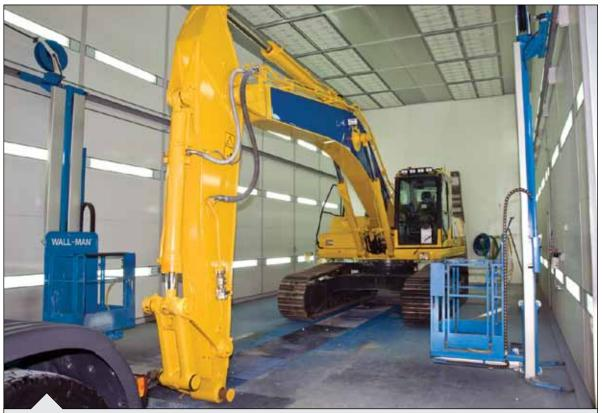
Also available are our Wall-Man units which are wall-mounted and can also telescope in and out from the wall for greater efficiency.
