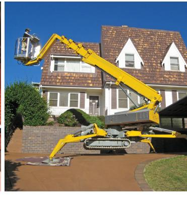
With features including dual power, auto-level, adjustable fly-jib etc, the 23 m Omme Spider Lift weighs only 3250 kg, making it the perfect machine for load-sensitive flooring. The soft non-marking rubber tracks are very gentle on fragile surfaces.
